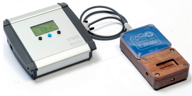
Figure 4: ELSOMA C10 flux density meter with measuring device
