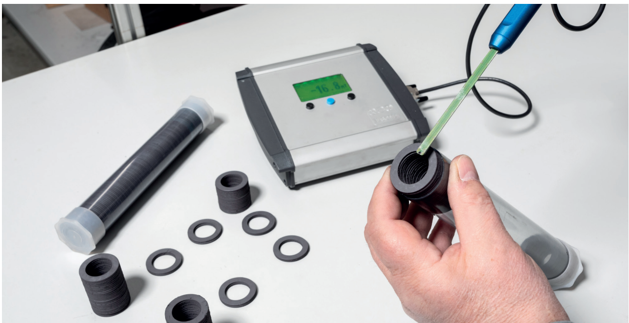
Figure 1: ELSOMA C10 flux density meter during incoming goods inspection of magnetic pole rings
