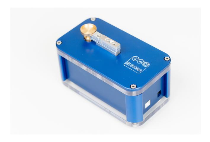
**Angle Based Magnetic Flux Density Meter A01**
